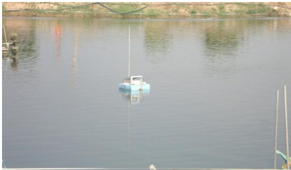
Dissolved Oxygen & Temperature continuous monitoring through GPRS
